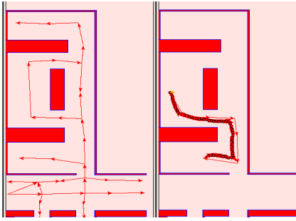
Figure 8. The figure's left side shows the topological map of an environment, the right side shows the path generated by a potential fields approach combined with the Dijkstra algorithm
