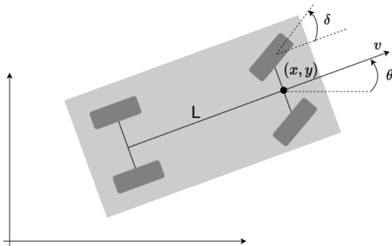
$$\begin{aligned}\dot{x} &= v \cos(\theta + \delta) \\ \dot{y} &= v \sin(\theta + \delta) \\ \dot{\theta} &= \frac{v}{L} \sin(\delta)\end{aligned}$$
